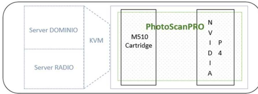
Figure 2 – PhotoScan Pro on low power server with GPU
